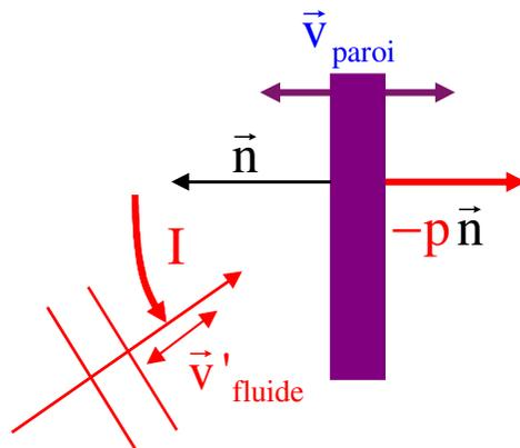
$$\bar{\sigma}_{\text{paroi}} \circ \vec{n} = -p \vec{n}$$
